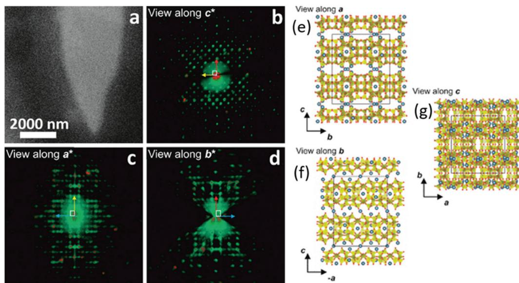
**Fig. 16** (a) STEM images of a cowlesite particle embedded in amorphous ice. (b) Projection of the reconstructed 3D ED data: (b) along  $c^*$ , (c) along  $a^*$ , and (d) along  $b^*$ . (e–g) The determined crystal structure of cowlesite along the three main crystallographic directions. The colour code for the atoms are: Si/Al in yellow, O atoms in red, and Ca atoms in blue. (Reprinted with permission from ref. 95. Copyright © 2020 American Chemical Society.)
