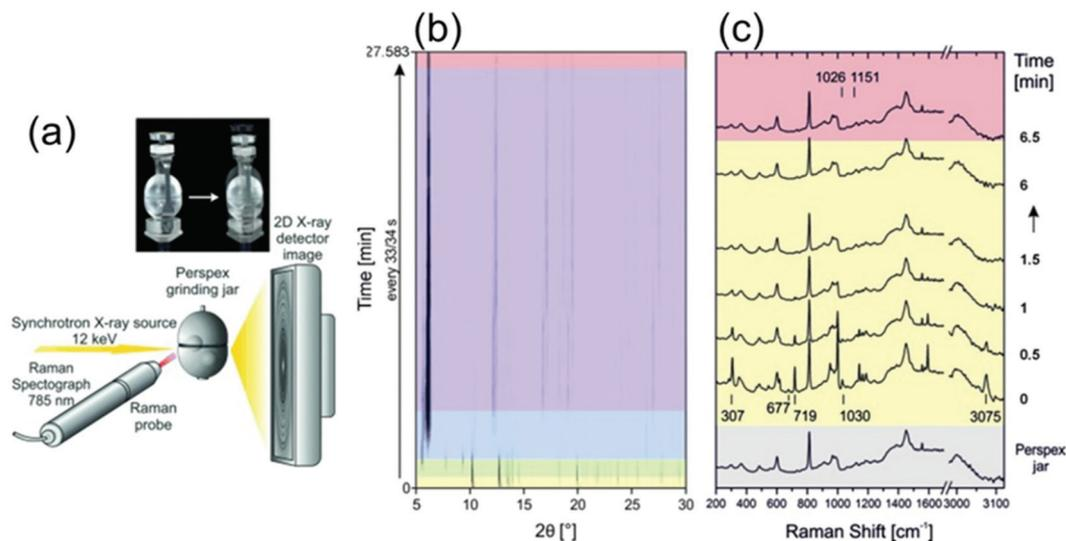
**Fig. 2** (a) A schematic representation of the experimental setup for recording Raman and XRPD data simultaneously during mechanochemical processes. (b) *In situ* synchrotron XRPD data and (c) simultaneously collected Raman spectra collected during the mechanochemical synthesis of  $\text{CoPhPO}_3 \cdot \text{H}_2\text{O}$ . (Reprinted with permission from ref. 37. Copyright © 2015 WILEY-VCH Verlag GmbH & Co. KGaA, Weinheim.)
