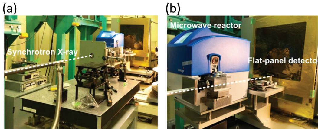
**Fig. 6** Photographs of the experimental setting for *in situ* X-ray total scattering measurements at BL08 W (SPRING-8). The photographs show the beam path through the vias (a) and the position of the vial fixed in the microwave reactor (b). Scattering data were recorded every 60 s. (Reprinted with permission from ref. 57. Copyright © 2017, American Chemical Society.)
