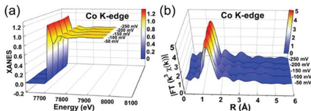
**Fig. 28** *In situ* XAS experiments of Co-SAS/HOPNC: (a) XANES and (b) FT-EXAFS spectra measured at the Co K edge at different potentials. (Reprinted with permission from ref. 135. Copyright © 2018. Published under the PNAS license.)
