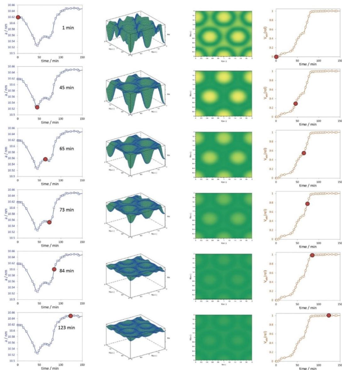
**Fig. 9** Left graphs represent the change of the unit cell parameters with adsorption time, the 3D and 2D representations of the electron densities are shown in the centre, and the relative volume adsorbed is plotted in the right column. The red dots indicate unit cell parameters and  $V_{\text{ads}}(\text{rel})$  at the respective time intervals. (Reprinted with permission from ref. 65. Copyright © 2020 American Chemical Society.)
