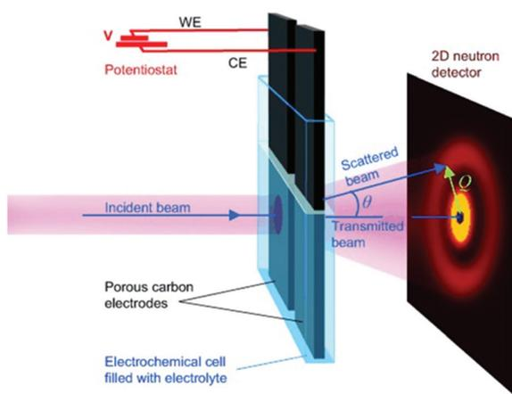
**Fig. 11** Experimental setup for *in situ* studies of ion adsorption on the surface of microporous carbon electrodes. (Reprinted with permission from ref. 69. Copyright © 2013 WILEY-VCH Verlag GmbH & Co. KGaA, Weinheim.)
