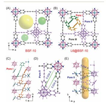
Fig. 2 Porous structure of BSF-10. (A) Generation of two kinds of pores by asymmetrical interpenetration. (B) L6 included in the large Pore I. (C) The packing mode of L6 in Pore I. (D and E) Structure of Pore II in two directions highlighting the closest B-H···H-B distance after subtracting the two van der Waals radii of hydrogen.
