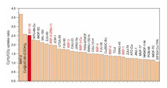
Fig. 6 Comparison of the C<sub>2</sub>H<sub>2</sub>/CO<sub>2</sub> uptake ratios at 298 K and 1 bar among BSF-10 and other well-performing materials in the context of C<sub>2</sub>H<sub>2</sub>/CO<sub>2</sub> separation by a thermodynamic mechanism.
