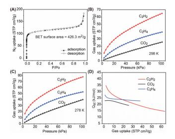
Fig. 4 (A) N<sub>2</sub> adsorption and desorption isotherms of BSF-10. (B and C) Single component adsorption isotherms of C<sub>2</sub>H<sub>2</sub>, CO<sub>2</sub> and C<sub>2</sub>H<sub>4</sub> on BSF-10 at 298 and 278 K. (D) Adsorption heats of C<sub>2</sub>H<sub>2</sub>, CO<sub>2</sub> and C<sub>2</sub>H<sub>4</sub> on BSF-10.
