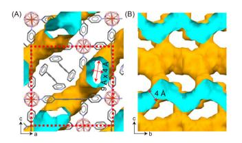
Fig. 3 Voids and pore windows of BSF-10 generated by a probe with the radius of 1.2 Å seen along (A) b-axis and (B) a-axis. The pore window dimensions are determined after subtracting the two van der Waals radii of hydrogen.
