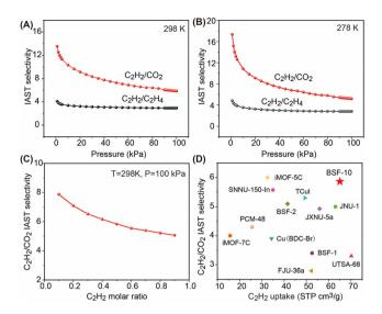
Fig. 5 (A and B) IAST selectivity of C<sub>2</sub>H<sub>2</sub>/CO<sub>2</sub> and C<sub>2</sub>H<sub>2</sub>/C<sub>2</sub>H<sub>4</sub> at 298 and 278 K. (C) IAST selectivity of C2H2/CO2 with different C2H2 molar ratios. (D) Comparison of the C<sub>2</sub>H<sub>2</sub> uptakes and C<sub>2</sub>H<sub>2</sub>/CO<sub>2</sub> selectivity among BSF-10 and others well-performing MOFs.
