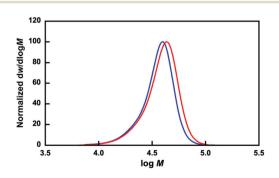
Fig. 3 Molecular weight distributions (normalized to peak height) of  $P(OEGMA-co-MEO_2MA)$  (blue line) and  $P(OEGMA-co-MEO_2MA)-b-PMPC$  (red line).
