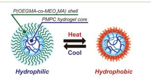
Fig. 8 Schematic illustration of the morphology of PMPC core-shell microgels and their temperature-responsive behaviour.
