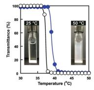
Fig. 7 Changes in transmittance (650 nm) of a PMPC core-shell microgel dispersion in water (●) and an aqueous P(OEGMA-co-MEO<sub>2</sub>MA) solution (O) as a function of temperature. (Inserted photos: PMPC coreshell microgel dispersion at 25 °C and 50 °C.)
