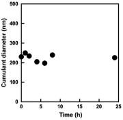
Fig. 5 Changes in cumulant diameter of water droplets of W/O emulsion in the continuous chloroform phase as a function of time after sonication for 3 min. The concentration of P(OEGMA-co-MEO<sub>2</sub>MA)-b-PMPC was 100 mg mL<sup>-1</sup> (relative to water dispersed phase).
