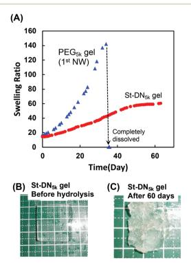
**Fig. 6** (A) Time course of swelling ratio during degradation test for 4-arm-PEG/PEG-DA ( $1^{\text{st}}$  NW) gel and St-DN gel in PBS (pH = 7.4) at 37 °C. (B) and (C): photographs for St-DN gel before hydrolysis test and after 60 days, respectively.
