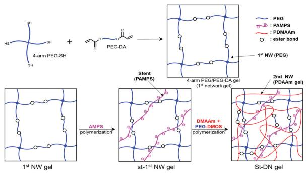
Scheme 1 Synthesis of St-DN gel comprising 4-arm PEG/PEG-DA as the first NW, linear PAMPS as the stent, and PDMAAm/PEG-DMOS as the second NW.
