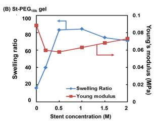
Fig. 4 Effect of stent concentration on the swelling ratios and Young's moduli of the (A) St-PEG<sub>5k</sub> and (B) St-PEG<sub>10k</sub> gels.
