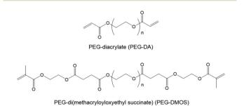
Fig. 1 Structures of the cross-linkers used in this study: PEG-DA and PEG-DMOS
