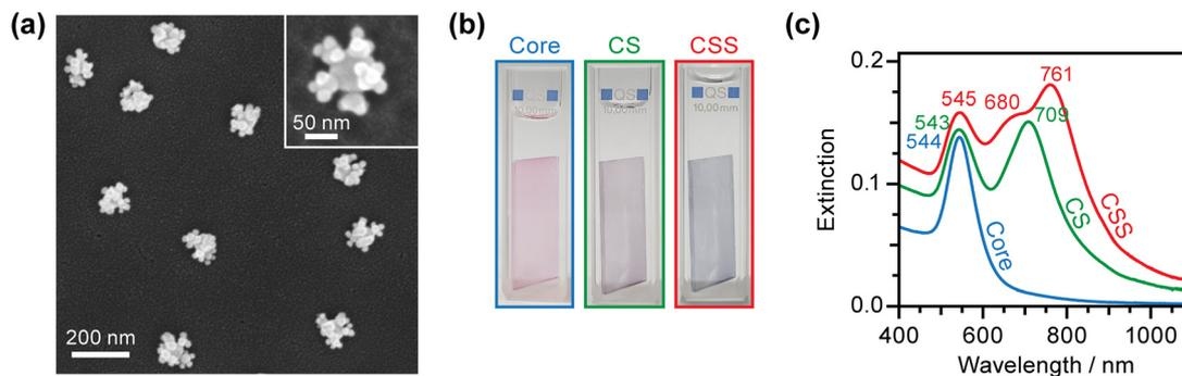
**Fig. 2** Structural and optical characteristics of CSS nanoassemblies. (a) Representative SEM image (inset: a magnified view) of CSS nanoassemblies with C8DT as linkers. (b) Photographic images and (c) UV-vis spectra of the Core, CS, and CSS with C8DT as linkers.
