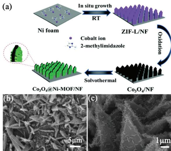
**Fig. 3** (a) Schematic illustration of the preparation of  $\text{Co}_3\text{O}_4@\text{Ni-MOF}/\text{NF}$ . (b and c) SEM images of the as-prepared  $\text{Co}_3\text{O}_4@\text{Ni-MOF}/\text{NF}$ . Reprinted with permission from ref. 57, Copyright 2021, Royal Society of Chemistry.
