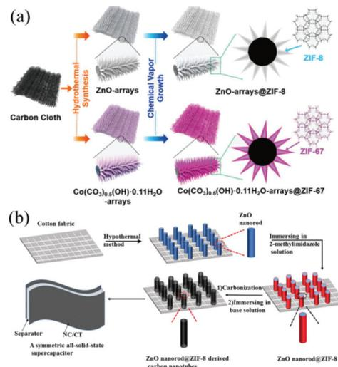
**Fig. 5** (a) Scheme showing the synthetic process of  $\text{ZnO}@ZIF-8$  and  $\text{Co}(\text{CO}_3)_{0.5}(\text{OH})\cdot 0.11\text{H}_2\text{O}@ZIF-67$  on CC. Reprinted with permission from ref. 63, Copyright 2018, American Chemical Society. (b) Schematic illustration showing the fabrication of  $\text{ZnO}@ZIF-8$  derived nanotubes. Reprinted with permission from ref. 64, Copyright 2018, Elsevier.
