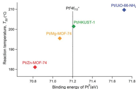
**Fig. 9** Relationship between catalytic activity (*i.e.* reaction temperature,  $T_{50}$ ) and electronic state of Pt NPs (*i.e.* binding energy of Pt<sup>0</sup> 4f<sub>7/2</sub>) of Pt/MOF catalysts. The black dotted line indicates the binding energy of bulk Pt<sup>0</sup> 4f<sub>7/2</sub>.
