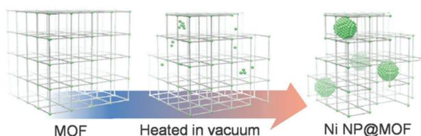
Fig. 2 Schematic illustration of the preparation of M/MOF composites through a partial decomposition method.
