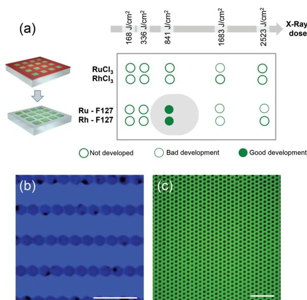
Fig. 4 (a) Summary of the results of the development for the two metal precursors Ru/Rh chlorides alone or in the presence of the block-copolymer (F127) as a function of exposure doses (b) and (c) false-colored optical micrographs of the developed Rh and Ru-based resists respectively (scale bar  $100 \mu m$ ).
