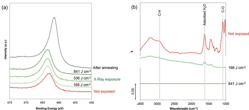
Fig. 2 (a) XPS spectra recorded in the Ru(3p) region on films exposed to different doses and annealed under a reducing atmosphere. (b) Evolution of the extinction coefficient  $k$  of a RuCl<sub>3</sub>/F127 film before and after exposure at different doses.
