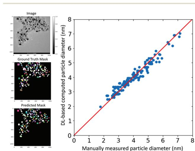
**Fig. 3** The left panel shows the TEM image, ground truth mask, and predicted mask. The right panel compares the manually measured particle diameter with the deep learning-based computed particle diameter.
