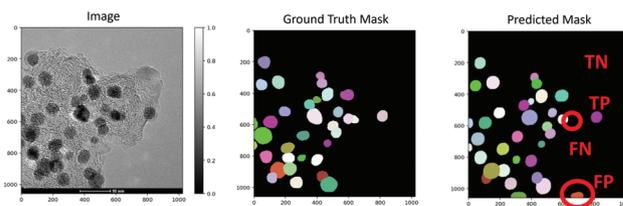
**Fig. 2** Demonstration of a TEM image along with the ground truth and predicted masks. Examples of true-positive (TP), true-negative (TN), false-positive (FP), and false-negative (FN) predictions are shown on the predicted mask.
