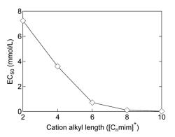
Fig. 2 Relationship between the alkyl chain length and EC  $_{\rm 50}$  of [C  $_n$  mim]Cl against IPC-81 cells.  $^{\rm 58,59}$
