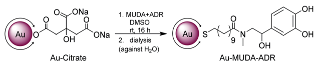
Scheme 3 Nanoparticle functionalisation in a ligand exchange reaction with the presynthesised catecholamine carrying ligands (MUDA-ADR or MUDA-NA), shown here with MUDA-ADR as an example.
