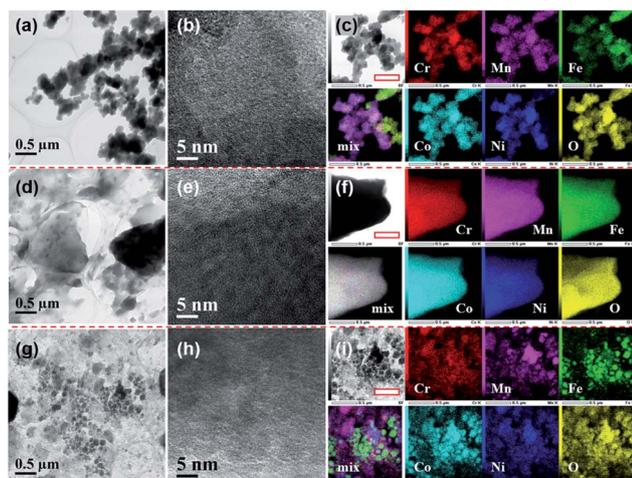
**Fig. 2** TEM, HRTEM and EDS maps of the HEH-1# as-synthesized products under different conditions. (a)–(c) EG-K, (d)–(f) EG-K/N, and (g)–(i) H<sub>2</sub>O-K/N. Scale bar in (c), (f), and (i) is 0.5 μm. Note: mix figure shows the overlapping Cr, Fe and Ni signals.
