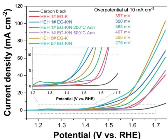
**Fig. 11** LSV curves of the HEH-1# and 5# as-synthesized products under various conditions, HEH-1# EG-K/N 200 °C- and 600 °C-annealed nanoparticles, and carbon black. Inset shows the expanded view for these curves.
