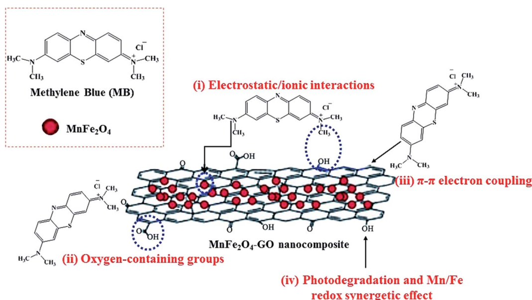
Fig. 25 Illustration of methylene blue (MB) adsorption mechanism on GO-MnFe 2 O 4 nanocomposites. This figure was adapted with permission from RSC Advances , 2018, 8, 12376–12389. 154
