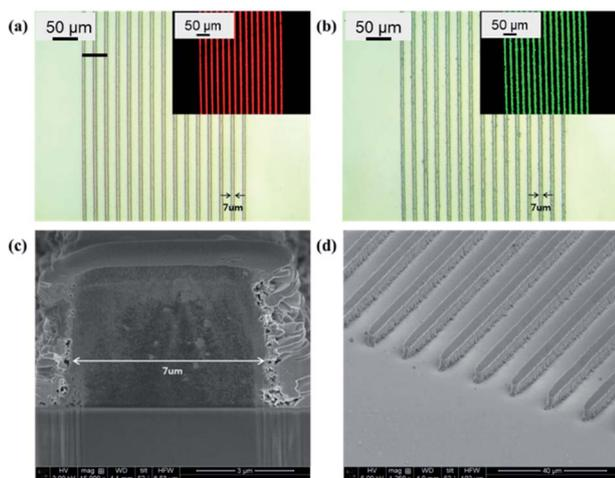
Fig. 4 Optical and fluorescence microscopy images (inset) of 7  $\mu\text{m}$  line patterns of red (a) and green (b) QDs, respectively. Cross-sectional (c) and birds-eye view (d). SEM images of the photolithographic line pattern shown in (a) and (b).
