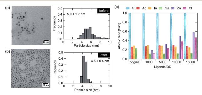
Fig. 4 TEM images and corresponding size distribution histogram of the AIGS QDs (a) before and (b) after ZnCl<sub>2</sub> addition at mole ratio of 10 000 ligands/QD. (c) Atomic ratio (sulfur basis) of the original AIGS QDs and the QDs after ZnCl<sub>2</sub> addition at mole ratios in the range of 1000–15 000 ligands/QD.
