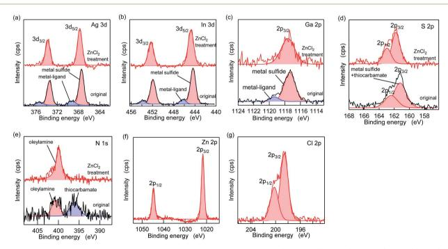
Fig. 5 XPS spectra of the pristine AIGS QDs (black lines) and the  $ZnCl_2$ -treated AIGS QDs (red lines). (a) Ag 3d, (b) In 3d, (c) Ga 2p, (d) S 2p, (e) N 1s, (f) Zn 2p, and (g) Cl 2p. (f) and (g) display the treated samples only.
