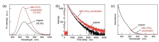
Fig. 3 (a) PL spectra, (b) PL decay curves, and (c) UV-vis absorption spectra of the AIGS QDs before (original) and after ZnCl<sub>2</sub> addition at a mole ratio of 10 000 ligands/QD
