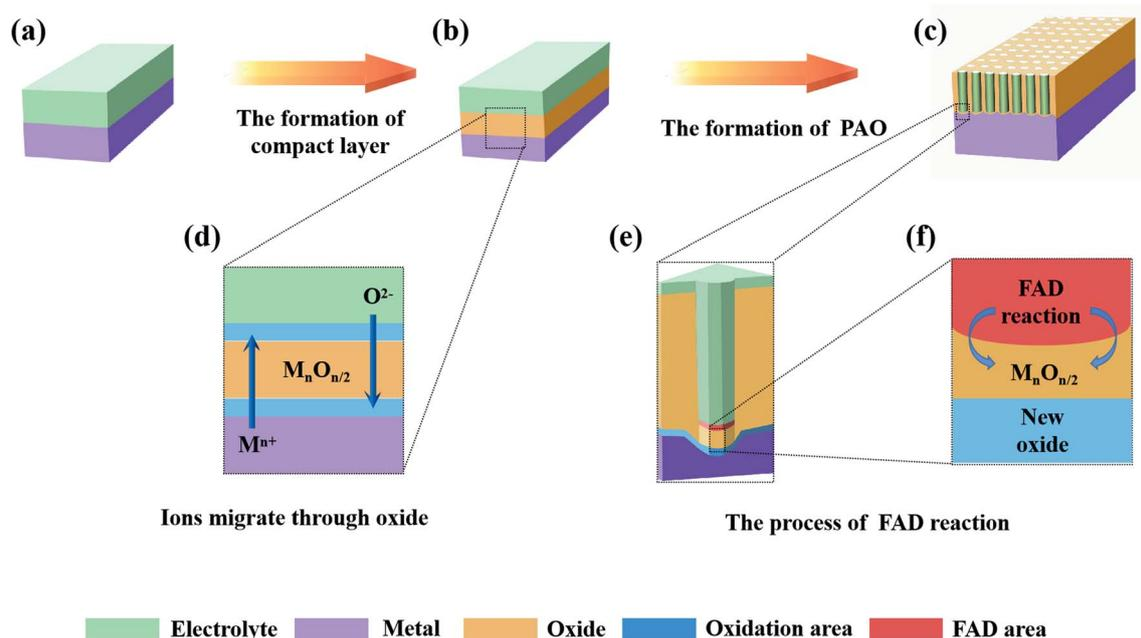
Fig. 2 Schematic of the mechanism of FAD theory.
