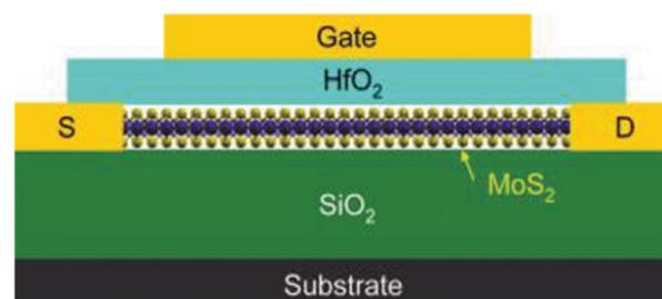
Fig. 25 Representation of the device structure of a MoS<sub>2</sub> transistor. Reprinted with permission from ref. 203 [Y. Yoon, K. Ganapathi and S. Salahuddin, *Nano Lett.*, 2011, **11**, 3768–3773]. Copyright 2011 American Chemical Society.
