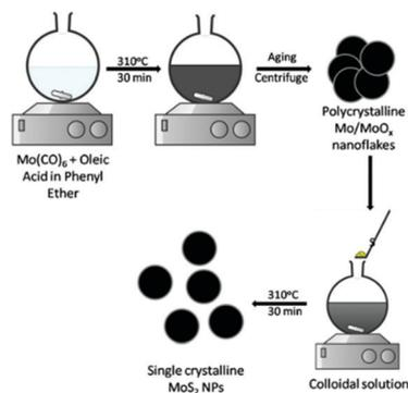
Fig. 9 Synthesis of ultra-small MoS<sub>2</sub> NPs using oleic acid.<sup>66</sup>
