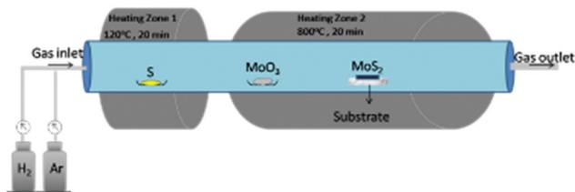
Fig. 11 Schematic diagram of the CVD system used to synthesise various sized MoS<sub>2</sub> nanoparticles by regulating the flow of gases.<sup>81</sup>
