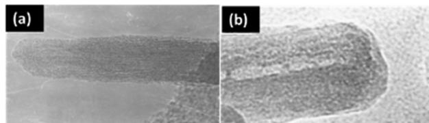
Fig. 14 MoSe<sub>2</sub> nanotubes obtained *via* decomposition of (a) MoSe<sub>3</sub> and (b) (NH<sub>4</sub>)<sub>2</sub>MoSe<sub>4</sub>. Reprinted with permission from ref. 94 [M. Nath and C. N. Rao, *Chem. Commun.*, 2001, 2236–2237]. Copyright The Royal Society of Chemistry.
