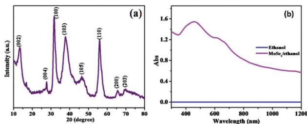
Fig. 6 XRD and UV-Vis spectra of 2H-MoSe<sub>2</sub>. Reprinted with permission from ref. 10 [N. T. Shelke and D. J. Late, *Sens. Actuators, A*, 2019, **295**, 160–168]. Copyright 2019, Elsevier.
