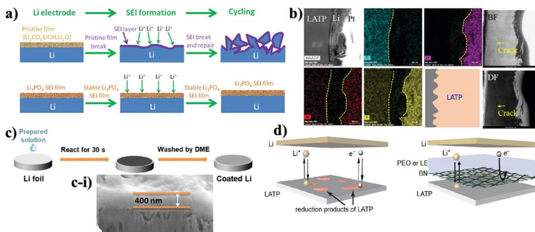
Fig. 2 Illustration of the deposition of various inorganic protective layers on LATP and their TEM and SEM images: (a) explanation of the role of the SEI layer;<sup>88</sup> (b) TEM-EDS of  $\text{Li}_3\text{PO}_4$  deposited LATP after 100 cycles;<sup>89</sup> (c) nanocomposite layer formation through the dropping of solution; (c-i) cross-sectional view of the nanocomposite layer on LATP;<sup>90</sup> (d) scheme of BN and polymer combined thin layer on LATP.<sup>91</sup>
