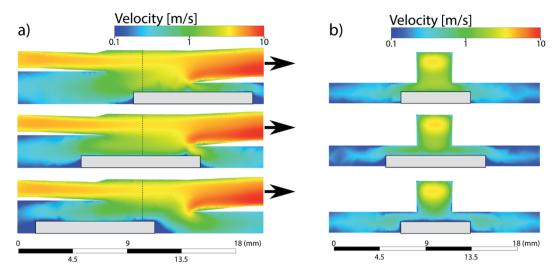
Fig. 6 Gas flow simulations for the PFAC for three different sample positions (grey) at a He flow rate of  $1.6 \, L \, min^{-1}$  and Ar flow rate of  $0.8 \, L \, min^{-1}$ . The sample (grey) is positioned  $0.8 \, mm$  below the opening. (a) Side view with the arrow representing the direction of the ICP. (b) Cross section at the dashed line from (a).
