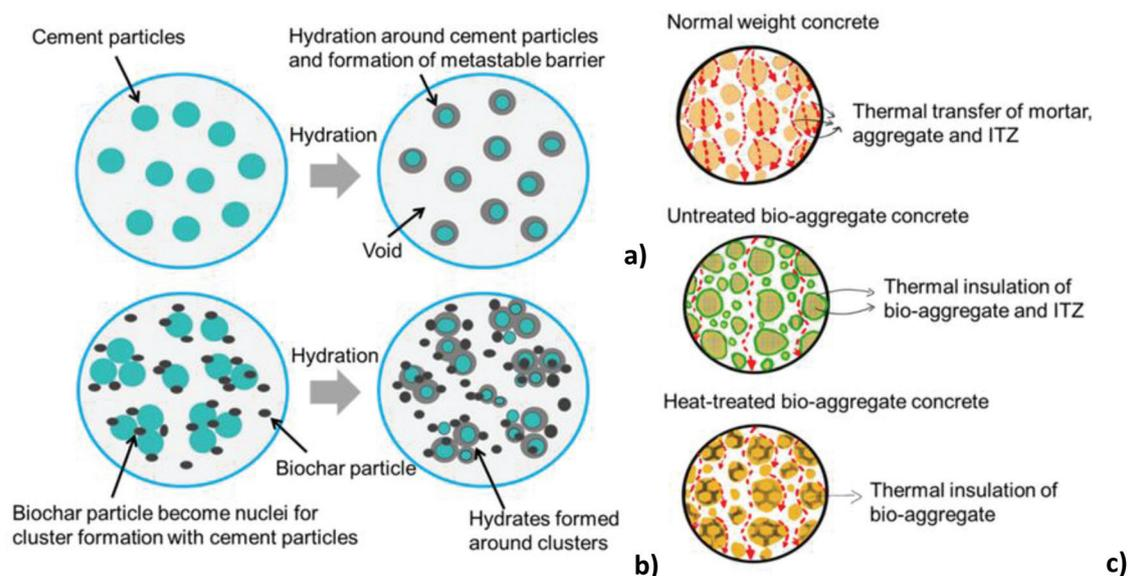
**Fig. 12** Schematics showing hydration product formation in (a) cement-only system and (b) system containing cement and biochar. (c) Thermal insulation mechanism of bio-based concrete (ITZ = interfacial transition zone). Reproduced from ref. 229 with permission from MDPI, copyright 2021.
