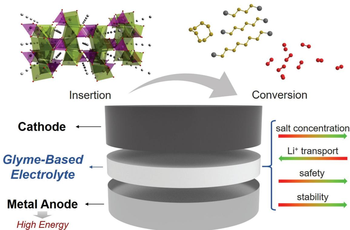
**Fig. 9** Schematic representation of the promising characteristics of glyme-based electrolyte solutions for application in lithium–metal batteries using insertion (e.g., olivine-based compounds) as well as conversion cathodes (e.g., S-based and O<sub>2</sub>-based electrodes); the typical relationship between LiX salt concentration, Li<sup>+</sup> transport properties, safety, and stability of the glyme-based solutions is also shown.
