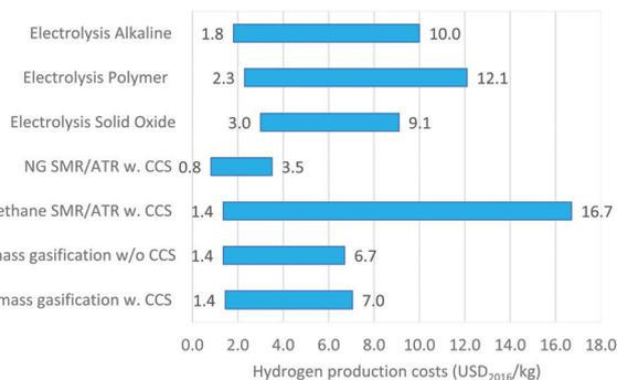
Fig. 3 Current reported cost ranges for selected hydrogen production technologies. Ranges based on values reported in Speirs *et al.*,<sup>131</sup> IEA,<sup>126</sup> Binder *et al.*,<sup>132</sup> Howes *et al.*,<sup>133</sup> Bauer *et al.*,<sup>134</sup> IEAGHG<sup>135</sup> and Parkinson *et al.*<sup>136,137</sup> and converted to 2016 USD per kg using an average 2016 USD/GBP exchange rate of 1.3552 and an average 2016 EUR/GBP exchange rate of 1.1068.
