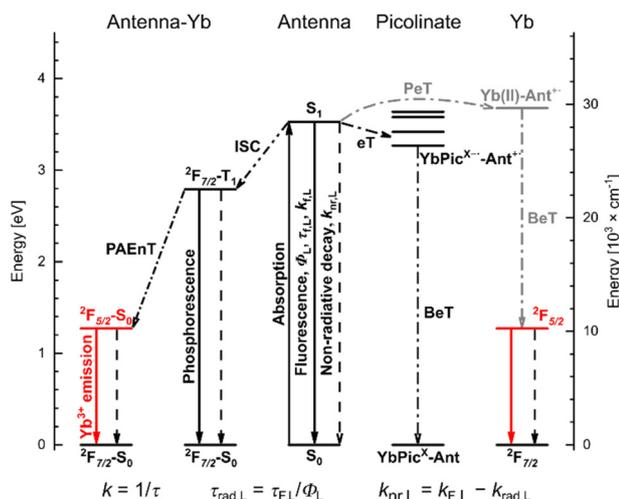
**Fig. 1** Competing sensitising and quenching processes in photoexcited **YbL<sup>X</sup>** complexes; solid and dashed lines indicate radiative and non-radiative processes, respectively.
