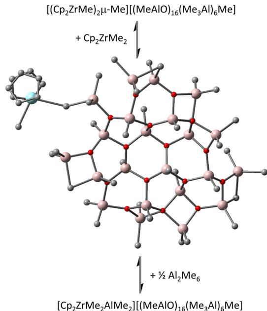
**Fig. 1** Equilibria involving contact ion-pair to form outer-sphere ion-pairs detected spectroscopically.<sup>15</sup> Zr in blue, Al in pink, O in red, C in grey, H omitted for clarity.
