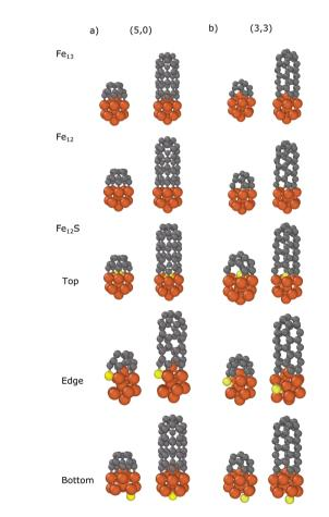
Fig. 4 Optimized structures of the carbon nanocap and CNT segment with chirality of (a) (5,0) and (b) (3,3) binding to  $Fe_{12}X$  (X = Fe, -, S)nanoparticles.
