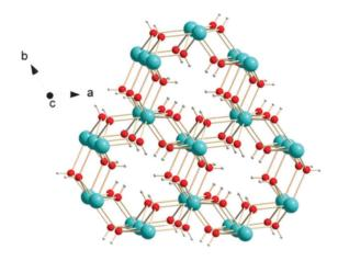
Fig. 6 Crystal structure of Gd(OH)<sub>3</sub>. Colour codes: Gd: cyan, O: red, H: white. Reproduced from ref. 70 with permission from the Royal Society of Chemistry.
