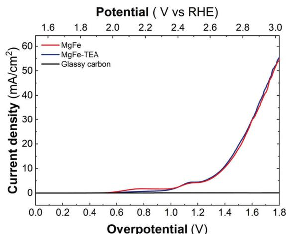
**Fig. 5** Linear sweep voltammetry (LSV) recorded at  $5 \text{ mV s}^{-1}$  in 1 M KOH solution by employing glassy carbon collectors for samples obtained with and without TEA, MgFe-TEA (blue) and MgFe (red), in comparison with the bare collector (black).
