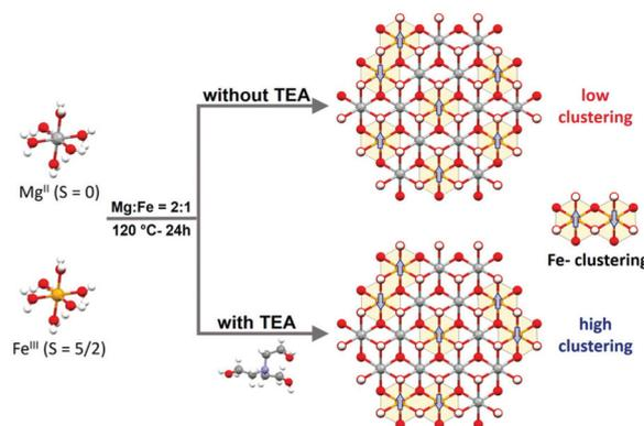
**Scheme 1** MgFe-based LDHs (Mg : Fe = 2 : 1 ratio) are synthesized hydrothermally with ammonia at 120 °C for 24 h. In the case of samples obtained through the TEA approach, a higher Fe-clustering degree is observed which triggers changes in the magnetic behaviour of the final MgFe-based LDHs, even at the same Mg : Fe = 2 : 1 ratio.
