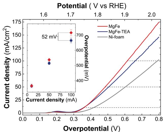
**Fig. 6** Linear sweep voltammetry (LSV) recorded at  $5 \text{ mV s}^{-1}$  in 1 M KOH solution for samples obtained with and without TEA, MgFe-TEA (blue) and MgFe (red), in comparison with an Ni-foam collector (gray). The inset shows the extracted overpotential at 10, 50, and  $100 \text{ mA cm}^{-2}$  for both samples, MgFe-TEA (blue) and MgFe (red).
