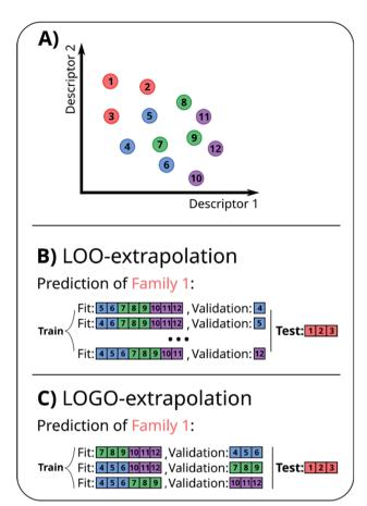
Fig. 2 (A) Example of a small 2D database with 12 points split among four families, indicated by their color. (B) Representation of the LOOextrapolation to predict the values of 'Family 1', where the algorithm is trained with a LOO cross-validation. (C) Representation of our proposed LOGO-extrapolation to predict the values of 'Family 1', where the algorithm is trained to extrapolate to other families and is finally tested to extrapolate the values of that new family.
