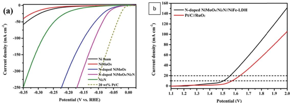
Fig. 115 Polarisation curves of Ni foam,  $\text{NiMoO}_4$ , N-doped  $\text{NiMoO}_4$ ,  $\text{Ni}_3\text{N}$  and N-doped  $\text{NiMoO}_4/\text{Ni}_3\text{N}$  heterostructure (a). LSV curves of N-doped  $\text{NiMoO}_4/\text{Ni}_3\text{N}/\text{NiFe-LDH}$  and commercial Pt/C// $\text{RuO}_2$  systems in 1.0 M KOH solution without iR correction (b). Reproduced with permission from ref. 1457. Copyright American Chemical Society 2020.
