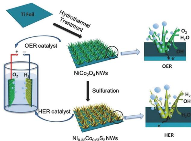
Fig. 45 Schematic illustration of the synthesis of  $\text{NiCo}_2\text{O}_4$  and  $\text{Ni}_{0.33}\text{Co}_{0.67}\text{S}_2$  nanowires, and the utilisation of these homologous Ni–Co based nanowires as OER and HER catalysts for water splitting. Reproduced with permission from ref. 796. Copyright Wiley 2015.
