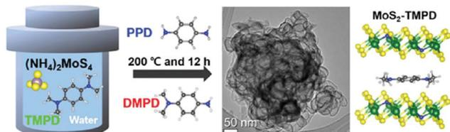
Fig. 140 One-step procedure of hydrothermal reaction for the synthesis of MoS<sub>2</sub> nanosheets that were intercalated with PPD, DMPD, and TMPD. Reprinted with permission from ref. 1708. Copyright Royal Society of Chemistry.
