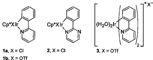
Fig. 124 Iridium catalysts for water oxidation. Reprinted with permission from ref. 1547 Copyright 2009. American Chemical Society.
