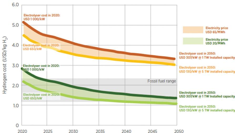
Fig. 172 Cost projections for green hydrogen production over time, as a function electrolyser capital cost and electricity price. Reproduced from IRENA.<sup>1903</sup>
