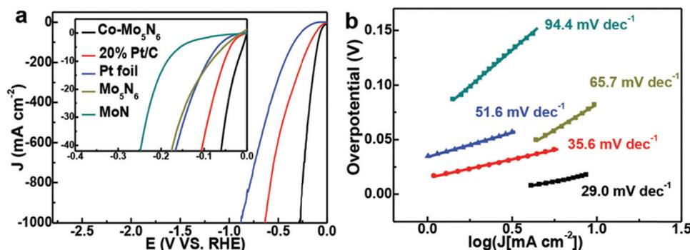
Fig. 68 Electrochemical measurements. (a) HER polarisation curves of the samples in  $1.0 \text{ M KOH}$ . (b) Corresponding Tafel plots. Reproduced with permission from ref. 1031. Copyright Wiley 2020.
