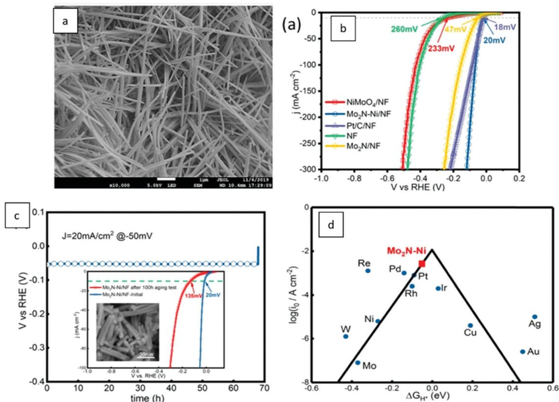
Fig. 116 SEM image of Mo<sub>2</sub>N–Ni/NF(a). LSV curves with iR correction in 1 M KOH (b). LSV curves of Mo<sub>2</sub>N–Ni/NF before and after a 100 h aging test, and the SEM image of Mo<sub>2</sub>N–Ni/NF after a 100 h aging test (c). Volcano plot of  $i_0$  as a function of  $\Delta G_{H^*}$  for Mo<sub>2</sub>N–Ni and some typical reported electrocatalysts (d). Reproduced with permission from ref. 1458. Copyright American Chemical Society 2020.
