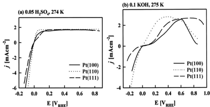
Fig. 18 Polarisation curves for hydrogen evolution/oxidation on Pt(*hkl*), with scan rate of 20 mV s<sup>-1</sup>, in (a) acid and (b) alkaline media. Reproduced with permission from ref. 409 (copyright MDPI 2020), 410 (copyright American Chemical Society 1997),<sup>412</sup> (copyright RSC 1996).
