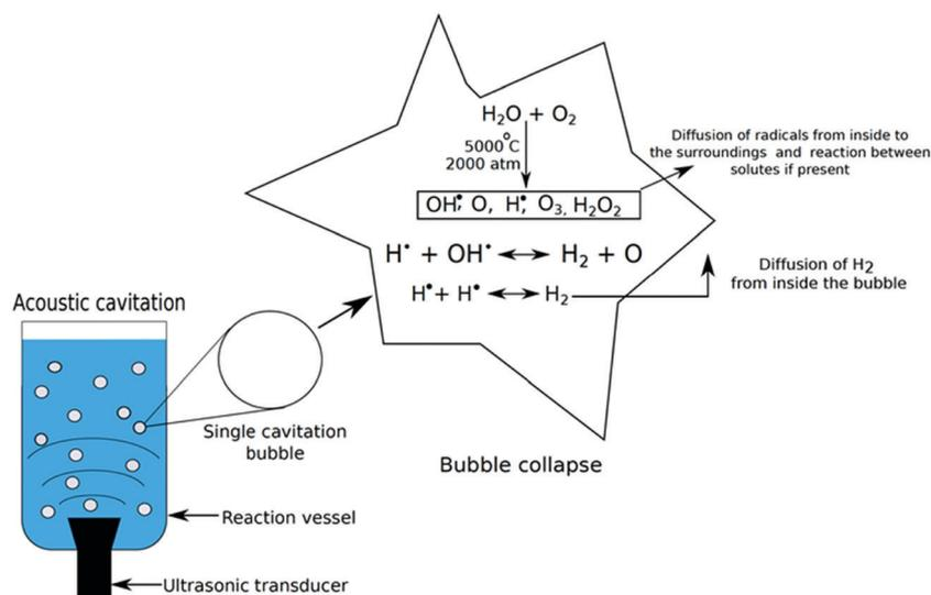
Fig. 147 Production of sonolysis species by acoustic cavitation.<sup>1846</sup>
