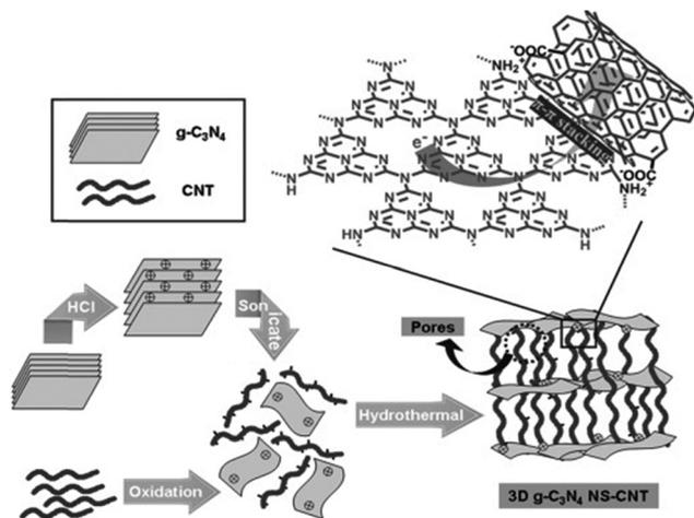
Fig. 100 Fabrication of the 3D g-C<sub>3</sub>N<sub>4</sub> NS-CNT porous composite. Reproduced with permission from ref. 1410. Copyright Wiley 2014.
