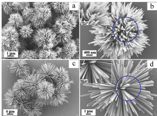
Fig. 23 SEM images of dandelion-like- (a and b) and urchin-like  $\alpha$ -MnO<sub>2</sub> (c and d). Reproduced with permission from ref. 509. Copyright Elsevier 2017.
