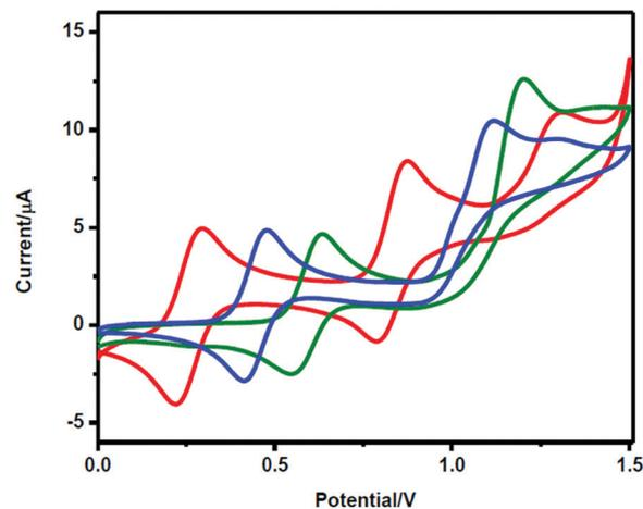
Fig. 131 Water oxidation in the presence of  $\text{Co}(\text{tpc})\text{Py}_2$  (red),  $\text{Co}(\text{tdfc})\text{Py}_2$  (blue) and  $\text{Co}(\text{tpfc})\text{Py}_2$  (green) in acetonitrile on adding 4.8% water. Reprinted with permission from ref. 1577 Copyright 2020. American Chemical Society.
