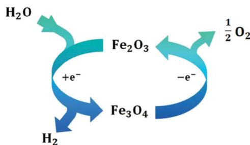
**Scheme 4** A cyclic process ensures electrocatalytically initiated splitting of water mediated through two different oxide species. Reproduced with permission from ref. 1328. Copyright Royal Society of Chemistry 2020.
