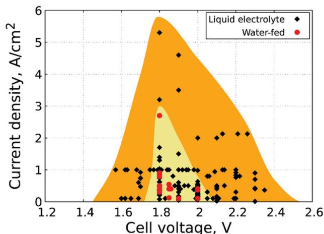
Fig. 12 Performance summary of AEMWEs: comparison of current densities achieved at cell voltages in the 1.5–2.4 V range, extracted from different polarisation curves with different feed types. Yellow and orange areas represent AEMWE performance data with (KOH addition) and without liquid electrolyte (pure water). Operating temperature ranges from 22 to 90 °C. Main design parameters, operating conditions and underlying sources are provided in Tables S3 and S4 (ESI<sup>†</sup>).
