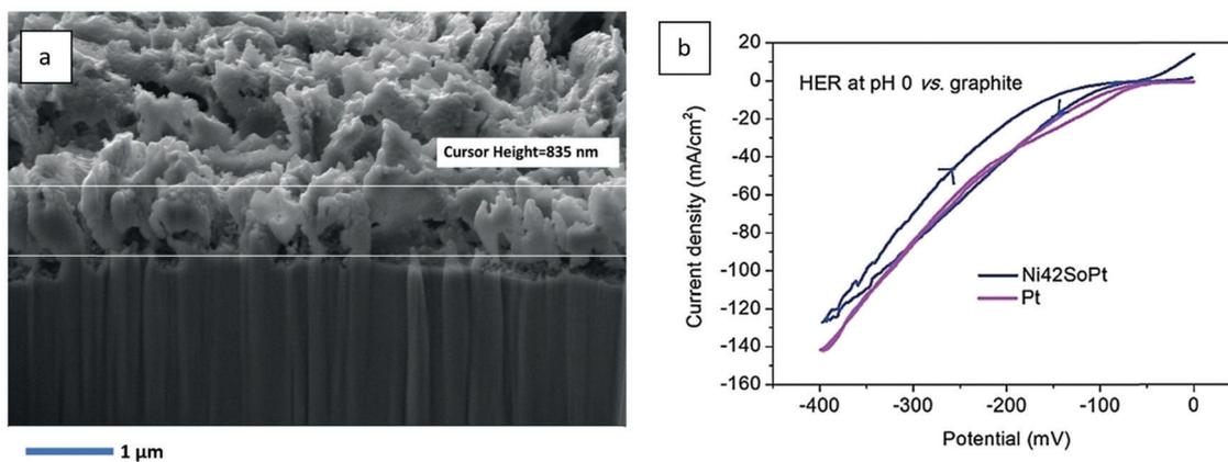
Fig. 106 (a) SEM photograph showing the cross-section of the Ni<sub>42</sub>/Pt interface (Pt thickness ~800–900 nm); the Pt loading is 1.8 mg cm<sup>-2</sup>. (b) comparison of the HER performances of Pt and Ni<sub>42</sub>SoPt at pH = 0. Reproduced with permission from ref. 1269. Copyright Wiley 2019.
