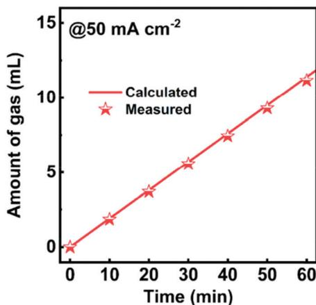
Fig. 154 Theoretically calculated and experimentally measured  $\text{O}_2$  amounts for NCFPO/CaCC as a function of time in the NaCl + KOH electrolyte. Reproduced with permission from ref. 1858. Copyright ACS 2020.
