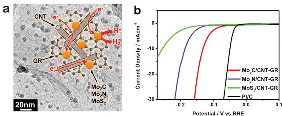
Fig. 61 (a) Schematic illustration of Mo<sub>2</sub>C-, Mo<sub>2</sub>N-, and MoS<sub>2</sub>-nanoparticles anchored on carbon nanotubes (in turn) attached to graphene and the corresponding discharging of H<sup>+</sup> ions leading to HER. (b) Polarisation curves derived from the nanoparticle-CNT-graphene hybrid electrocatalyst. Measurements were performed in 0.5 M H<sub>2</sub>SO<sub>4</sub>. Reproduced with permission from ref. 985. Copyright American Chemical Society 2014.
