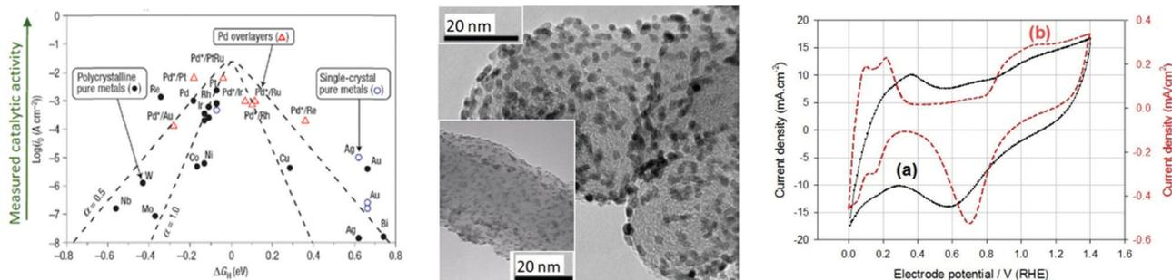
Fig. 104 (a) Volcano plots of  $j_0$  vs. M-H bond energy. (b) SEM micrographs of nano-Pt/C electrocatalysts for the HER. (c) Cyclic voltammograms measured (a) on metallic Pt in 1 M H<sub>2</sub>SO<sub>4</sub>; (b) *in situ* at the cathode of a PEM water electrolysis cell. Reproduced with permission from ref. 1431 Copyright Elsevier 2014.
