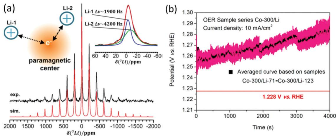
Fig. 92 (a)  ${}^7\text{Li}$  MAS NMR spectrum of (as-prepared) Co-300/Li recorded at 11.7 T and a MAS frequency of 25.0 kHz, showing a broad, asymmetric spinning sideband pattern characteristic of a strong electron-Li dipolar interaction. (b) Averaged chronopotentiometry curve based on 53 samples of the sample series Co-300/Li (blacksquares) with standard error bars (magenta). Reproduced with permission from ref. 1324. Copyright American Chemical Society 2018.
