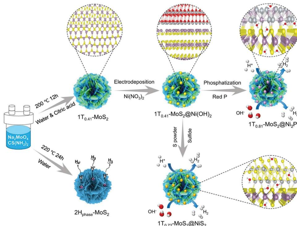
Fig. 82 Schematics of the  $1T_{0.72}$ - $\text{MoS}_2$ @ $\text{NiS}_2$  and  $1T_{0.81}$ - $\text{MoS}_2$ @ $\text{Ni}_2\text{P}$  synthesis steps. Reproduced with permission from ref. 1185 Copyright Nature Publishing 2021.
