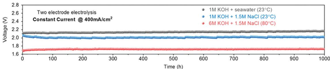
Fig. 153 Durability tests (1000 h) recorded at a constant current of  $400 \text{ mA cm}^{-2}$  of the seawater-splitting electrolyser under 1 M KOH + real seawater at room temperature and 6 M KOH electrolyte at  $80^\circ \text{C}$ , respectively. (h) Reproduced with permission from ref. 1857. Copyright PNAS 2019.
