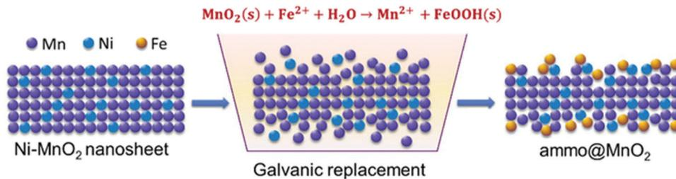
Fig. 25 Process of the surface-guided formation of ammo@MnO<sub>2</sub> via the galvanic replacement reaction. Reproduced with permission from ref. 514 Copyright Wiley 2017.
