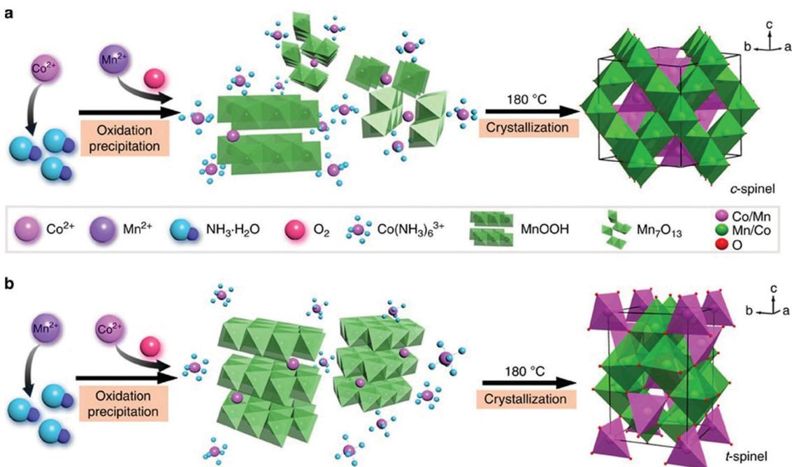
Fig. 40 Schematic synthesis of cubic (a) and tetragonal (b) spinel phases, involving two steps of oxidation precipitation and crystallisation. Reproduced with permission from ref. 707. Copyright Nature Publishing 2015.
