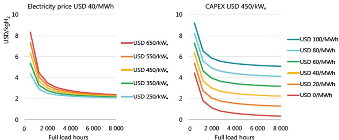
Fig. 170 Hypothetical future levelised cost of hydrogen production from electrolyzers as a function of capital cost (left) and electricity cost (right). Calculations assume a discount rate of 8% and efficiency of 69% (LHV). Reproduced from IEA.<sup>1889</sup>
