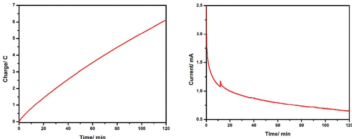
Fig. 132 The charge vs. time and current vs. time plots obtained from chronoamperometric measurements at an applied potential of 1.5 V for two hours to the Co(tpfc)Py<sub>2</sub>-loaded Nafion film. Reprinted with permission from ref. 1577 Copyright 2020 American Chemical Society.
