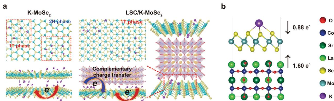
Fig. 34 (a) Schematic of the atomic structure and charge transfer effect for K-MoSe<sub>2</sub> and LSC/K-MoSe<sub>2</sub>. Complementary charge transfer in LSC/K-MoSe<sub>2</sub> can modulate the electronic structure of MoSe<sub>2</sub>, increasing the 1T-MoSe<sub>2</sub> ratio in the heterostructure. (b) Charge transfer from K and LSC to MoSe<sub>2</sub> in the optimised LSC/K-MoSe<sub>2</sub> heterostructure. Reproduced with permission from ref. 684. Copyright Nature Publishing 2021.
