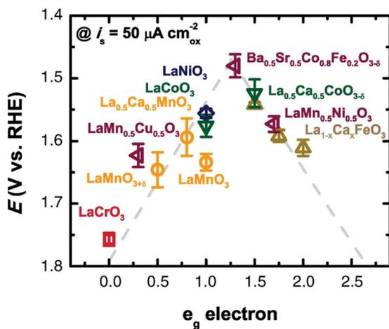
Fig. 30 Relation between observed OER activities of perovskites (ABO<sub>3</sub>) and the number of e<sub>g</sub> symmetry electrons of the transition metal (B in ABO<sub>3</sub>). Reproduced with permission from ref. 611. Copyright AAAS 2011.
