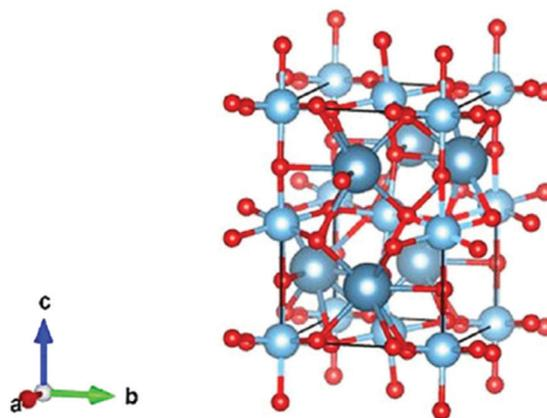
Fig. 31 Schematic structure of CaTiO<sub>3</sub> perovskite. Reproduced with permission from ref. 580. Copyright Wiley 2019.
