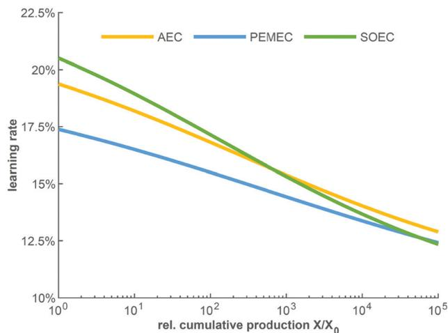
Fig. 163 The development of experience rates for electrolysis stack modules as a function of cumulative production. Reproduced from Böhm *et al.*<sup>1910</sup>
