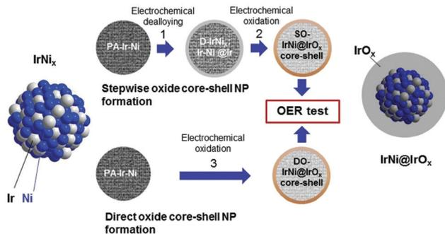
Fig. 102 Overview of the protocol used for the synthesis of SO-IrNi@IrO<sub>x</sub> and DO-IrNi@IrO<sub>x</sub> hybrid core-shell nanoparticle catalysts. Reproduced with permission from ref. 1429. Copyright. RSC 2014.
