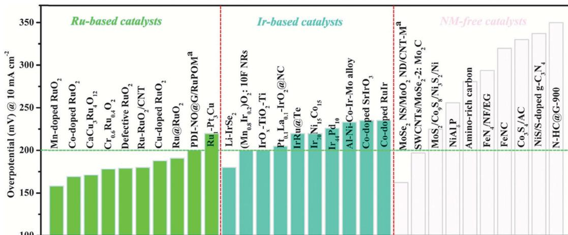
Fig. 20 Comparison of OER overpotentials at  $10 \text{ mA cm}^{-2}$  for the ten most promising catalysts in each category (Ir-, Ru- and PGM-free based catalysts) in acidic media. (a: the overpotential @  $20 \text{ mA cm}^{-2}$ ). Reproduced with permission from ref. 419. Copyright Elsevier 2020.
