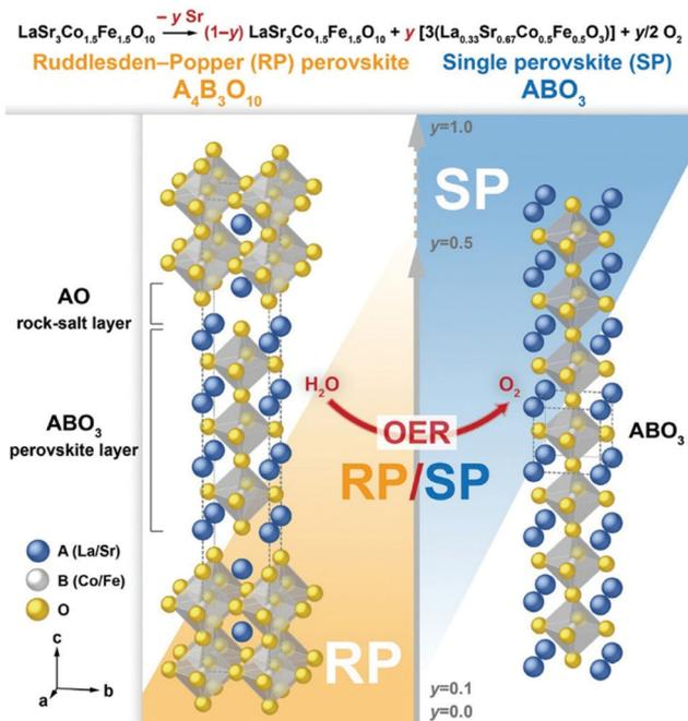
Fig. 35 Design of RP/SP composites. Schematic for the RP/SP composites showing RP and SP phase crystal structures. The unit cell of the SP structure is duplicated along the *c*-axis, to suggest a difference in the material's dimensionality, that is, 2D for RP versus 3D for SP. Reproduced with permission from ref. 596. Copyright Wiley 2021.
