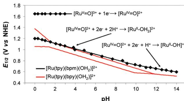
Fig. 120 Plots of  $E_{1/2}$  (V vs. NHE) vs. pH for the Ru(v/iv) and Ru(iv/iii) redox couples of [Ru(tpy)(bpm)(OH<sub>2</sub>)]<sup>2+</sup> and for the Ru(III/II) and Ru(III/II) redox couples of [Ru(tpy)(bpy)(OH<sub>2</sub>)]<sup>2+</sup> in aqueous solution (I) 0.1 M; (T) 298 K; glassy carbon working electrode). Reprinted with permission from ref. 1479 Copyright 2008. American Chemical Society.
