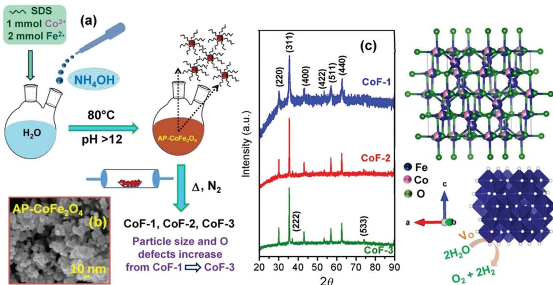
Fig. 47 (a) Schematic illustration of the formation of AP-CoFe<sub>2</sub>O<sub>4</sub> through the coprecipitation method followed by thermal treatment under N<sub>2</sub> to obtain CoF-1, CoF-2, and CoF-3. (b) Field-emission (FE) SEM image of AP-CoFe<sub>2</sub>O<sub>4</sub>. (c) XRD patterns of CoF-1, CoF-2, and CoF-3 NPs. Reproduced with permission from ref. 811. Copyright Wiley 2020.
