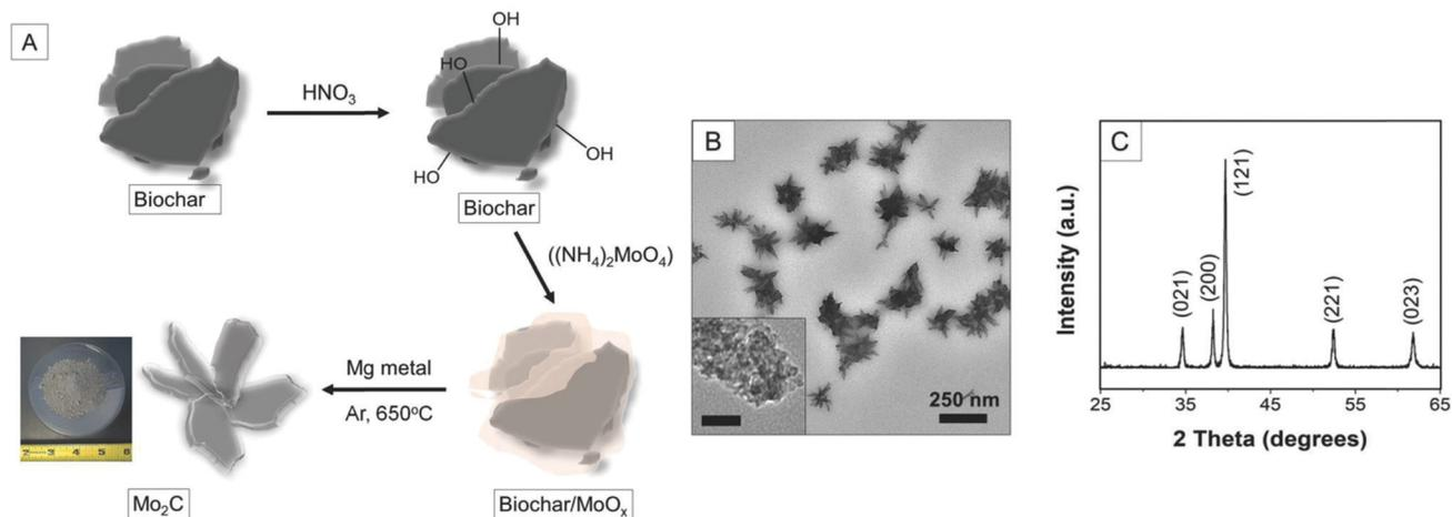
Fig. 63 (A) Schematic representation of synthesis of  $\text{Mo}_2\text{C}$  nanostructures. (B) TEM image (inset: scale bar = 25 nm) and (C) the powder XRD pattern of  $\text{Mo}_2\text{C}$  derived from biochar. Reproduced with permission from ref. 1002. Copyright Wiley 2018.
