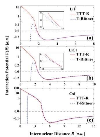
Fig. 4 Comparison of the damped TTT-R with the undamped T-Rittner potential curves for LiF, LiCl and Csl. In the attractive region the potentials are virtually identical. Small differences start to occur at small distances as the potentials become positive. The TTT-R potentials curves display the expected behavior at small distances, whereas the T-Rittner potentials bend over and become negative.
