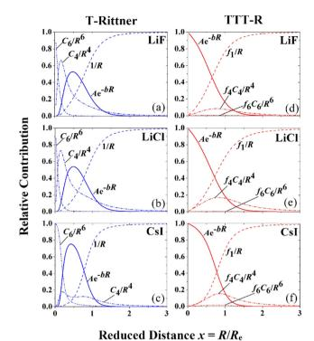
Fig. 3 Diagram showing the effects of damping on the relative contributions to the overall T-Rittner and TTT-R potentials. The frames (a-c) display the relative contributions of the repulsive Born-Mayer term (sold line) and the attractive Coulomb, induction and dispersion terms (broken lines) to the undamped T-Rittner model. Frames (d-f) show the corres-
