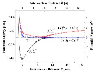
Fig. 1 Ab initio potential curves of LiCl showing the avoided crossing between the ionic  $X^1\Sigma^+$  state and the  $A^1\Sigma^+$  covalent state.<sup>24</sup> In a collision of an alkali atom with an halogen atom at the avoided crossing the outer electron of the alkali atom transfers to the halogen atom thereby producing two oppositely charged ions which attract each other and form a strong ionic bond
