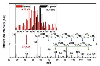
Fig. 9 Photoionization mass spectrum of products in syngas conversion over  $ZnCrO_x$  by SVUV-PIMS at 9.72 eV. The insets display the signals of m/z = 42.01 (ketene) and m/z = 42.05 (propene) detected at 9.72 and 11.40 eV, respectively.<sup>16</sup> Adapted and reproduced with permission from AAAS.
