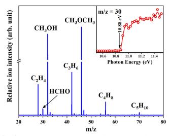
Fig. 10 Photoionization mass spectrum of the products of the MTH process recorded at 11.0 eV. The inset shows the PIE spectrum of the product with m/z 30.<sup>17</sup> Reaction conditions: HSAPO-34 was used as a catalyst; the reaction temperature was 450 °C; the pressure was 2 Torr; the methanol weight hourly space velocity was 11.74  $g_{methanol}$   $g_{catalysts}^{-1}$   $h^{-1}$ . Adapted and reproduced with permission from Wiley-VCH Verlag GmbH & Co. KGaA. Weinheim.
