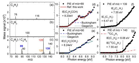
Fig. 6 Photoionization mass spectra and PIE curves of critical intermediates in the  $C_3H_3I/C_4H_2$  reaction. (a) 0.16%  $C_3H_3I$  and 99.84% Ar; (b) 16.64%  $C_4H_2$ and 83.36% Ar; (c) 0.16% C<sub>3</sub>H<sub>3</sub>I, 16.64% C<sub>4</sub>H<sub>2</sub>, and 83.20% Ar. All mass spectra were obtained at the photon energy of 8.5 eV. PIE curves for (d) m/z 89, (e) m/z 90, (f) m/z 139, and (g) m/z 140.66 Reproduced with permission from the American Chemical Society.
