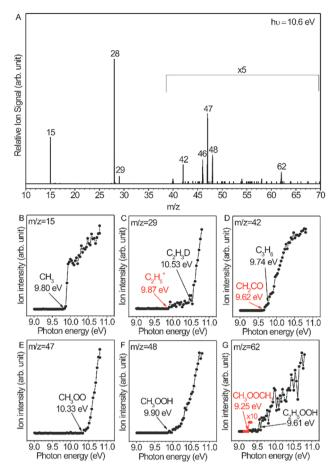
Fig. 8 (A) Gas-phase products of the OCM reaction catalysed by 5.6%-Li/ MgO at 750 °C, the mass spectrum was acquired at the photon energy of 10.6 eV and with a catalyst bed of 137 mm obtained from the sampling nozzle of the mass spectrometer. (B-G) Photoionization efficiency spectra of the reactive intermediates.<sup>72</sup> Reproduced with permission from the American Chemical Society.
