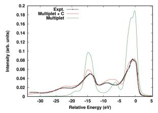
Fig. 12 Fe 2p XPS of  $\alpha$  Fe<sub>2</sub>O<sub>3</sub> calculated within the multiple + C approach (red) compared to the multiplet-only spectrum (green), and experimental results (black crosses). Reprinted figure with permission from [J. J. Kas, J. J. Rehr and T. P. Devereaux, Ab initio multiplet plus cumulant approach for correlation effects in X-ray photoelectron spectroscopy, 2021, https:// arxiv.org/abs/2107.10409].
