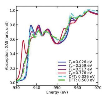
Fig. 7 L-Edge XAS of Cu metal at various electronic temperatures. Note the sharp peak appearing below the X-ray edge as function of increasing electronic temperature, which occurs due to the broadening of the Fermi function. Reprinted figure with permission from [T. S. Tan, J. Kas and J. Rehr, *Phys. Rev. B*, 2021, **104**, 035144], Copyright (2022) by the American Physical Society.
