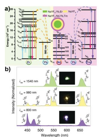
**Fig. 2** (a) Proposed multiple excited state absorption and energy transfer mechanism in Nd<sup>3+</sup>, Yb<sup>3+</sup>, Er<sup>3+</sup>, and Tm<sup>3+</sup>-codoped UCNC.<sup>76</sup> (b) Upconversion emission spectra of UCNCs shown in (a) and the corresponding photo of UCNC films excited using  $\lambda_{\rm ex}$  = 800, 980 and 1540 nm laser excitation.<sup>76</sup> Reprinted with permission from ref. 76. Copyright 2020, Nature Publishing Group.
