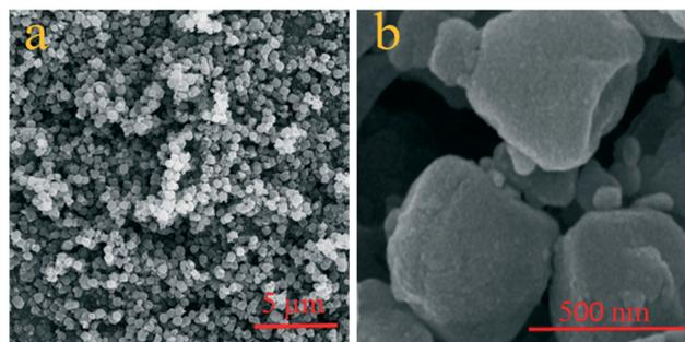
**Fig. 4** SEM images of CLN@ZIF-8 in a) bulk and b) magnified form.
