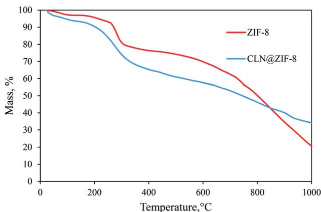
**Fig. 5** Thermal graphs of ZIF-8, CLN and CLN@ZIF-8.
