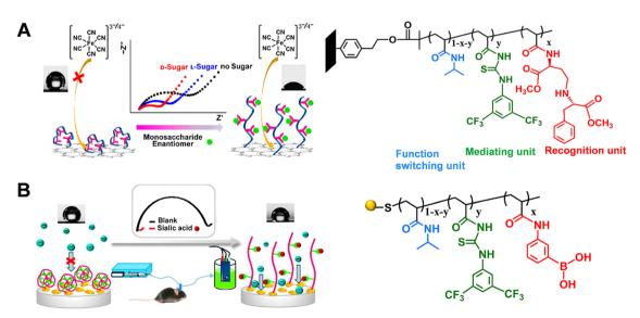
Fig. 8 Schematic illustration of the electrochemical biosensor based on stimuli-responsive polymers for measurement of (A) monosaccharide enantiomer and (B) sialic acid in live mouse brain. Reproduced with permission from ref. 81 and 82. Copyright 2016 and 2017, American Chemical Society.
