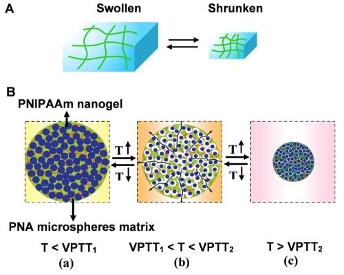
Fig. 6 (A) Schematic illustration of reversible volume phase transition of hydrogel. (B) The rapid response process of nanocomposite smart hydrogel upon heating-up or cooling-down. Reproduced with permission from ref. 76. Copyright 2012, Elsevier.
