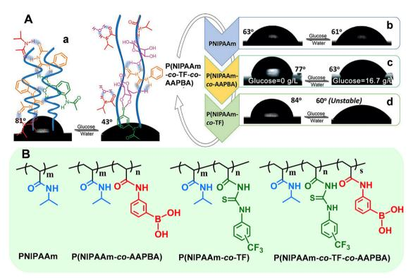
Fig. 4 (A) Surface wettability of the polymer films deposited on flat silicon wafers: (a) P(NIPAAm-co-TF-co-AAPBA), (b) PNIPAAm, (c) P(NIPAAm-co-TF-co-AAPBA), (b) PNIPAAM, (c) P(NIPAAM-co-TF-co-AAPBA), (d) PNIPAAM, (e) P(NIPAAM-co-TF-co-AAPBA), (e) PNIPAAM, (e) PNI AAPBA), and (d) P(NIPAAm-co-TF). (B) Chemical structures of the above stimuli-responsive polymers. Reproduced with permission from ref. 33. Copyright 2017, John Wiley and Sons.
