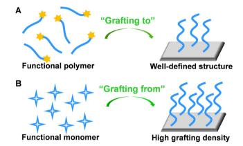
Fig. 5 Schematic illustration of preparation of stimuli-responsive polymer brush by (A) "grafting-to" and (B) "grafting-from" approaches.
