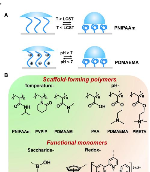
Fig. 2 (A) Schematic illustration of reversible conformation/wettability changes of (a) PNIPAAm induced by temperature and (b) PDMAEMA induced by pH. (B) Chemical structures of some common stimuli-responsive polymers and functional monomers.
