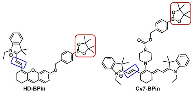
**Fig. 1** Chemical structures of **HD-BPin** and **Cy7-BPin**. Red box highlights  $\text{H}_2\text{O}_2$  and  $\text{ONOO}^-$  reactive aryl boronate motif. Blue box highlights  $\text{ONOO}^-$  reactive methine bridge.
