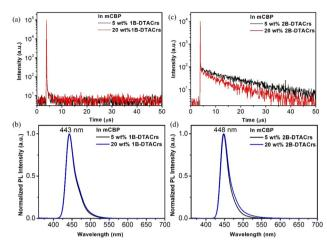
Fig. 4 Decay profiles and emission spectra of (a) and (b) 1B-DTACrs and (c) and (d) **2B-DTACrs** at different doping concentrations in mCBP ( $\lambda_{\rm exc}$  = 280 nm and 320 nm for time-resolved and steady-state emission, respectively)
