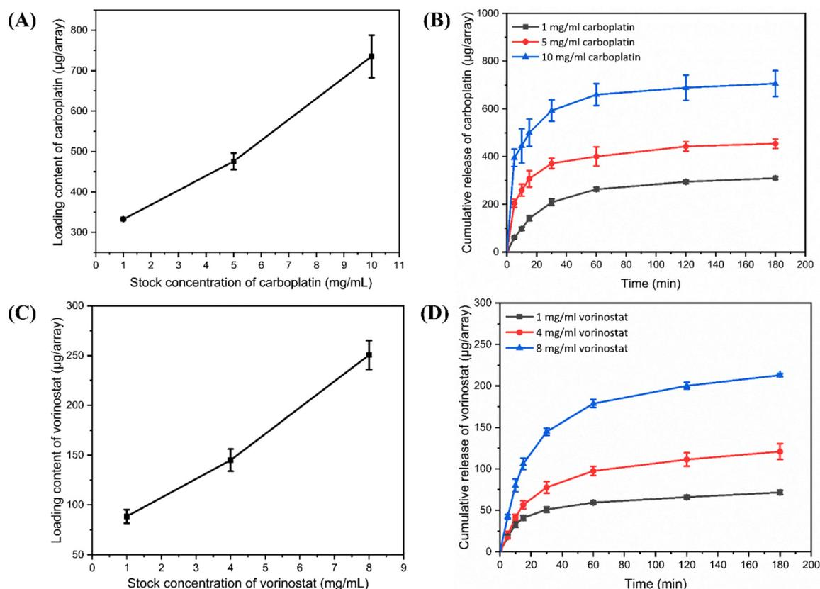
**Fig. 4** The total drug loading content of CBP@PF-MNP (A) and SAHA@PF-MNP (C) with different concentrations of the adsorbed solution. The drug release profile within 3 h of CBP@PF-MNP (B) and SAHA@PF-MNP (D) with different concentrations of the adsorption solution.
