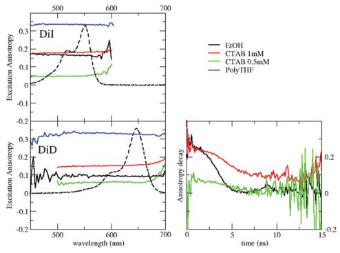
Fig. 3 Steady state (left) and time resolved (right) emission anisotropy of Dil (top) and DiD (bottom). Time resolved anisotropy of DiD was measured by exciting the sample at 590 nm and detecting emission at 675 nm.
