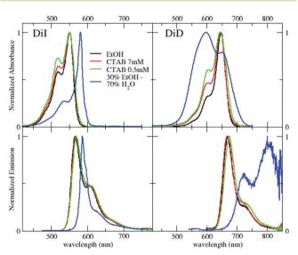
Fig. 2 Absorption (top) and emission (bottom) spectra of Dil and DiD (left and right panels, respectively) in different environments. Emission spectra of Dil and DiD were collected by exciting the samples at 495 nm and 600 nm, respectively (to minimize inner filter effects, 7 mM CTAB spectra were obtained with a 1.5 mm optical path cuvette).
