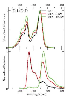
Fig. 4 Absorption and emission spectra (excitation wavelength: 495 nm) of solutions/suspensions of 1:1 Dil/DiD in different environments.
