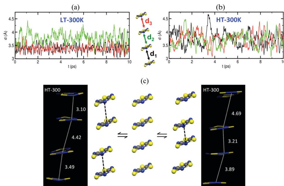
**Fig. 7** Time-resolved evolution of the distance between centroids of adjacent TTTA radicals in one of the columns (see  $d_1$  to  $d_3$  in a 4 radicals  $\pi$ -stack cluster model) of (a) LT-300 and (b) HT-300. (c) Regular  $\pi$ -stack of the HT polymorph (centre) results from the dynamic interconversion between two distorted stacks (left- and right-hand side). Examples of each distorted  $\pi$ -stack as extracted from the AIMD HT simulation at 300 K.
