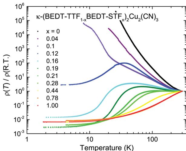
Fig. 3 DC resistivity of  $\kappa$ -[(BEDT-TTF) $_{1-x}$ (BEDT-STF) $_x$ ] $_2$ Cu $_2$ (CN) $_3$  for various substitution values  $x$  measured as a function of temperature along the highly conducting  $c$ -axis and normalized to the room-temperature values. The substitution spans the full range from the insulating  $x = 0$  to the metallic side.
