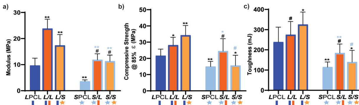
Fig. 4 Compressive mechanical properties were compared including (a)  $E$ , (b) CS, and (c) toughness; \* $p < 0.05$ , \*\* $p < 0.01$ , # $p > 0.05$ . Note: the black color-coded statistics are compared to the *LPCL* and light blue color-coded statistics are compared to *SPCL*.
