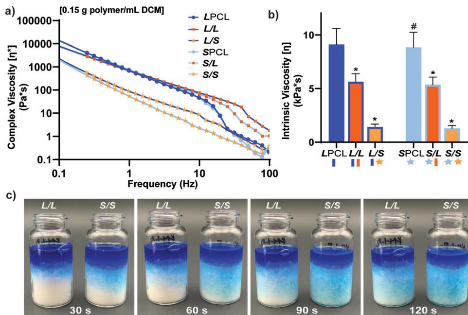
**Fig. 6** For scaffold precursor solutions: (a) Complex viscosity  $[\eta^*]$  versus frequency, (b) intrinsic viscosity (\* $p < 0.05$ , \*\* $p < 0.01$  compared to LPCL). (c) L/L and S/S semi-IPN macromer solution diffusion through a template using 15.0 g salt in a scintillation vial.
