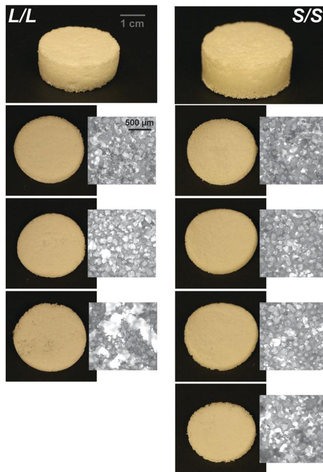
Fig. 7 Photos and optical microscopy (5x) of scaled-up, "large" *L/L* and *S/S* scaffolds ( $d \sim 24 \text{ mm}$ ) demonstrating superior macromer diffusion, and more uniform pores, for the *S/S* composition.
