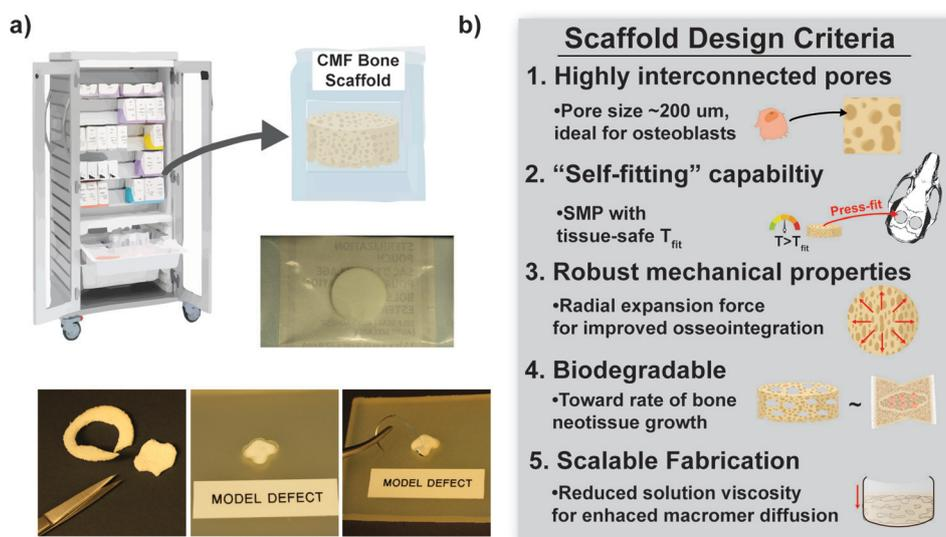
**Fig. 8** (a) The scaled-up, larger scaffold specimens ( $d \sim 24\text{ mm} \times t \sim 2\text{ mm}$ ) were able to be easily cut to custom defect geometries with scissors and could hold a suture. (b) The *S/S* semi-IPN (*i.e.* comprised of *star*-PCL-TA and *star*-PLLA) achieved five scaffold design criteria intended for an off-the-shelf surgical product to heal bone defects.
