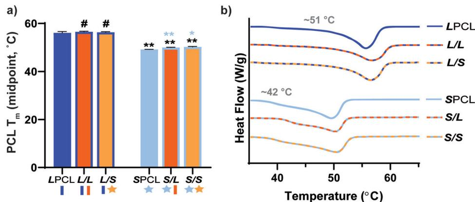
Fig. 2 (a) Midpoint  $t_m$  of PCL of scaffolds; \* $p < 0.05$ , \*\* $p < 0.01$ , # $p > 0.05$ . Note: the black color-coded statistics are comparisons to *LPCL* and blue color-coded statistics are comparisons to *SPCL*. (b) Representative thermogram for each scaffold composition.
