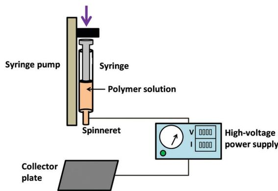
Fig. 2 A schematic illustration of the electrospinning process.
