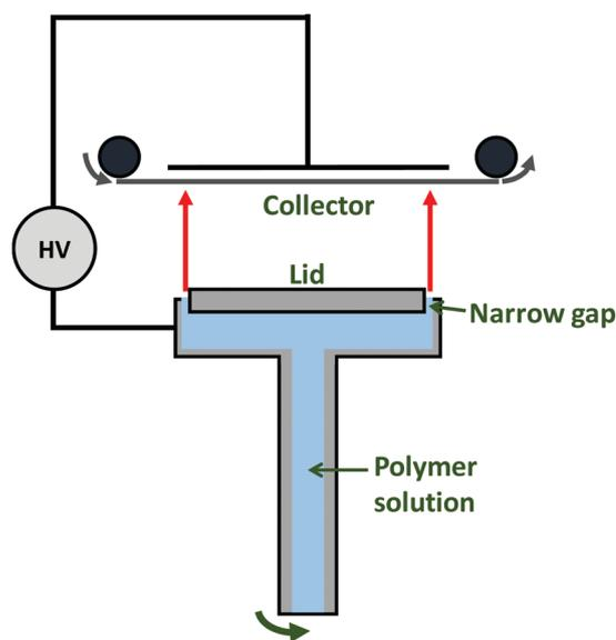
Fig. 10 Schematic diagram of the corona electrospinning apparatus developed by Molnar *et al.*<sup>117</sup>
