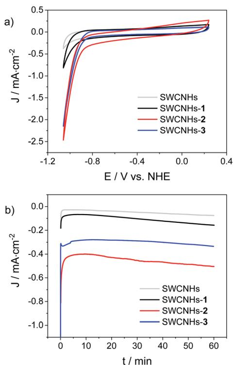
Fig. 3 (a) CV (scan rate of  $10 \text{ mV s}^{-1}$ ) and (b) chronoamperometry ( $-0.96 \text{ V vs. NHE}$ ) of SWCNHs electrodes ( $1.5 \text{ cm}^2$  surface area) functionalized with cobalt complexes 1–3 measured in  $1 \text{ M}$  phosphate buffer pH 7.4 (Pt as counter electrode, SCE as reference).
