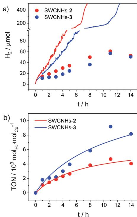
Fig. 4 (a) Theoretical (lines, from chronoamperometry, Fig. S27†) vs. experimental (dots, from gas chromatography) amount of hydrogen produced upon electrolysis at  $-0.96 \text{ V vs. NHE}$  of SWCNHs-2 and SWCNHs-3 electrodes ( $3.1 \text{ cm}^2$  surface area) in  $1 \text{ M}$  phosphate buffer  $\text{pH } 7.4$  (Pt as counter electrode, SCE as reference); (b) TONs of hydrogen production for SWCNHs-2 and SWCNHs-3 electrodes.
