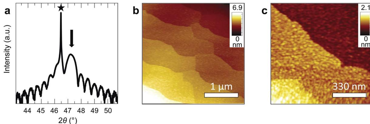
Fig. 1 (a) X-ray diffractogram of a 20 nm LaNiO<sub>3</sub> film on Nb:SrTiO<sub>3</sub>. The (002) substrate peak is marked with a star, the (002)<sub>pc</sub> film peak with an arrow. (b and c) Atomic force microscopy (AFM) of a 20 nm LaNiO<sub>3</sub> film with different magnification. AFM was performed after UHV transfer from the deposition tool to the analysis chamber.
