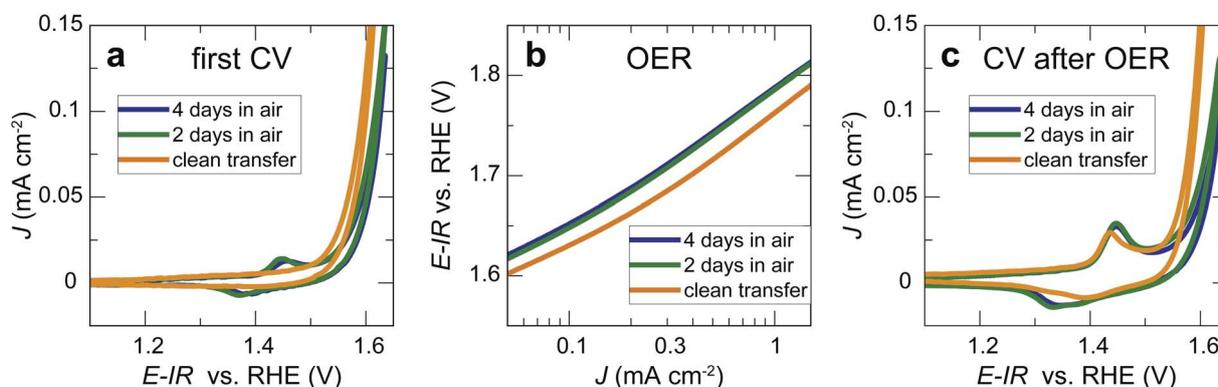
**Fig. 3** (a) First sweep during cyclic voltammetry in the Ni redox region with representative 20 nm LaNiO<sub>3</sub> thin film electrocatalysts. (b) Cyclic voltammetry in the OER potential regime. The average between anodic and cathodic sweep of the second cycle is shown. (c) First sweep during cyclic voltammetry in the Ni redox region after two sweeps to OER potentials. Scan rate was 10 mV s<sup>-1</sup> for all panels.
