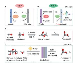
Scheme 1 Overview of hydrogen production and formic acid manufacturing. (a) Typical water electrolysis device. (b) Energy-efficient and value-added hydrogen production system in this work. (c) Industrial formic acid production. (d) Solar-assisted formic acid electrosynthesis in this work.
