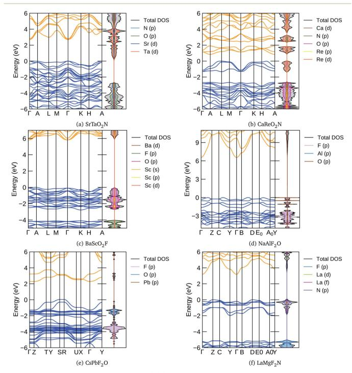
Fig. 5 The band structures and density of electronic states (DOS) of the lowest energy perovskite structures were calculated with the HSE06 functional for (a)  $SrTaO_2N$ , (b)  $CaReO_2N$ , (c)  $BaScO_2F$ , (d)  $NaAlF_2O$ , (e)  $CsPbF_2O$ , and (f)  $LaMgF_2N$ .
