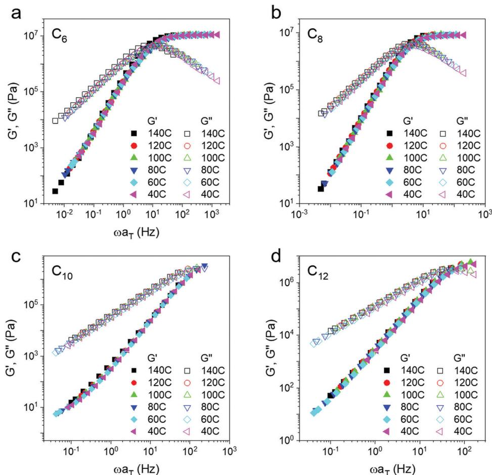
Fig. 3 Horizontally shifted master curves ( $T_{\text{ref}} = 140$  °C) of the networks. The high frequency rubbery modulus remains constant with increasing temperature, intermediate to expectations for permanent and dissociative dynamic networks.
