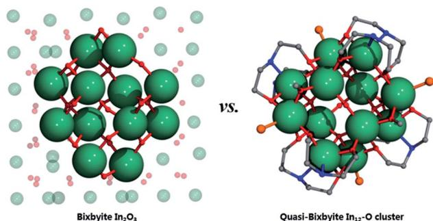
Fig. 2 Contrastive illustration of In–O connectivity in the bixbyte  $\text{In}_2\text{O}_3$  (left) and the  $\text{In}_{12}$ -oxo skeleton (right) of **InOC-1**. Atom color code: dark-green, In; red, O; blue, N; gray, C; orange, Cl. All H atoms have been omitted for clarity.
