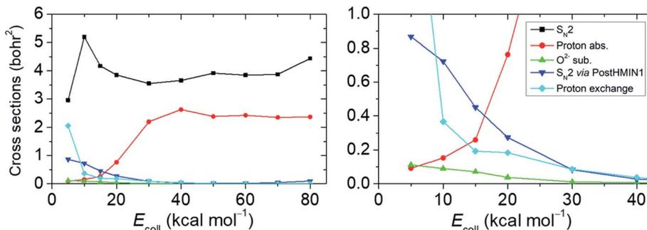
Fig. 3 Integral cross sections of the studied pathways at several collision energies. For the  $\text{OH}^- + \text{CH}_3\text{F}$  reaction, cross sections are determined in the range of 5–80  $\text{kcal mol}^{-1}$  collision energies for the reaction pathways of  $\text{S}_{\text{N}}2$ , proton abstraction, oxide ion substitution,  $\text{S}_{\text{N}}2$  occurring via the deep PostHMIN1 and proton exchange.
